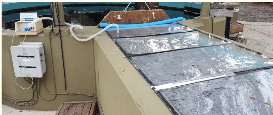
Figure 1: Plexiglass taped together and placed over transfer channel connecting medical pools. Condensation demonstrates the trapped warm air provided by the heated pool originating from the pool in the lower right corner of the picture (not shown). Nebulizer shown is commercial over the counter product readily available in pharmaceutical outlets.
