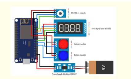
Figure 1: Circuitry of the Inspect used to measure the body temperature of sows.
