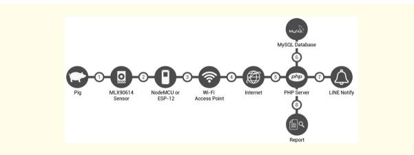
Figure 2: Systemic architecture of the measurement system used to measure the body temperature of sows.
