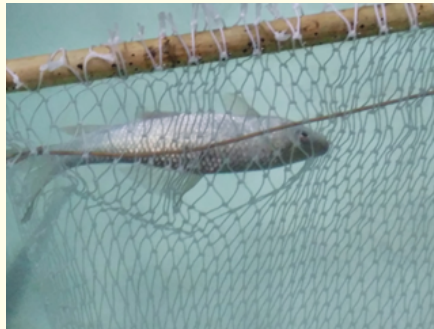
Figure 8: Cirrhinus mrigala entangled around the positive electrode of the central panel of electrified gill net.
