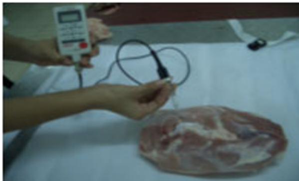
Figure 4: pH meter; inserting glass electrode in meat tissue.
