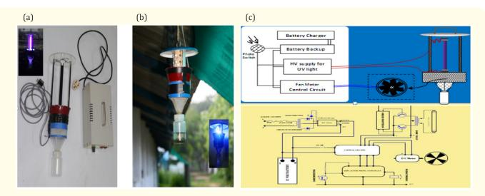
Figure 1: Light Trap (a) UV fluorescent light (b) UV LED (c) line diagram of light trap with the circuit.
