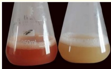
Figure 5: Adsorption and degradation of methyl orange by white rot fungi Schizophyllum commune (In broth).
