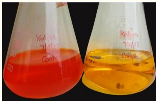
Figure 4: Adsorption and degradation of methyl orange by white rot fungi Schizophyllum commune (In broth).
