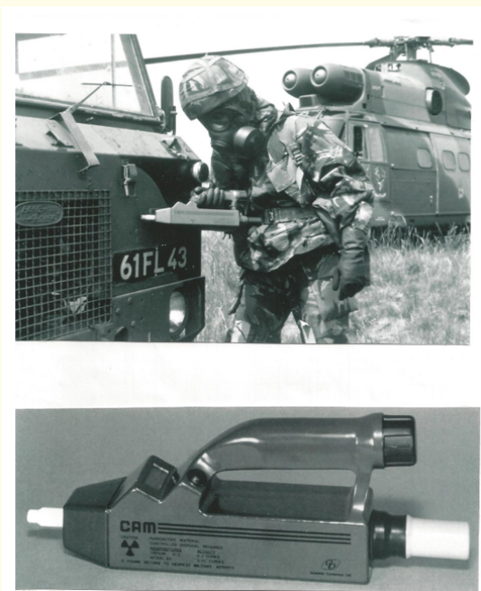
Figure 6: British soldier used CAM (Chemical Agent Monitor) for military exercise. The figure obtained from NATO document.
