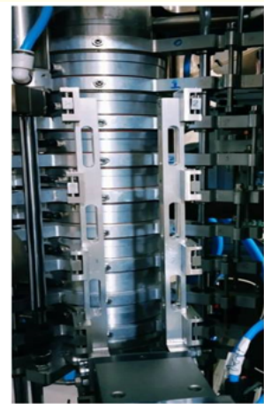
Figure 5: The closed and sandwiched isolator/ACI column.
