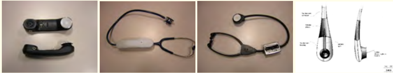
Figure 1: Several prototypes of the digital stethoscope that we developed.
