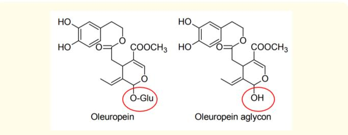
*Figure 3a and 3b:* Chemical structures of oleuropein and oleuropein aglycon. (Note the presence of the glutamate group in oleuropein but absence in the aglycon, as circled in figure 3a and 3b).
