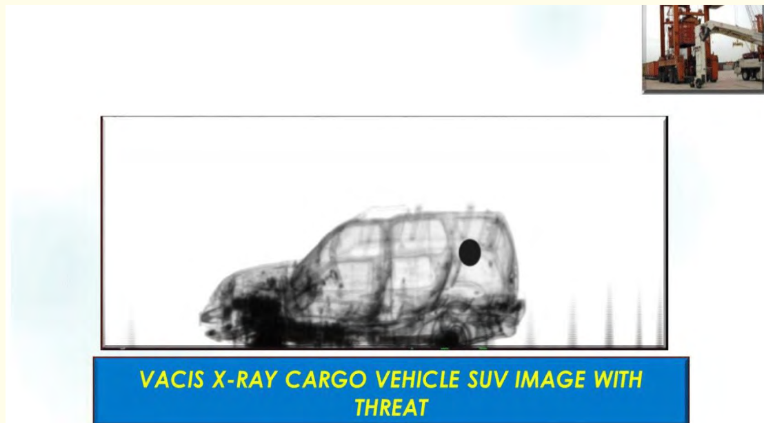
Figure 3: VACIS x-ray cargo vehicle SUV image with threat.
