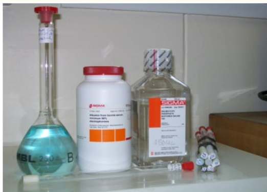
Figure 1: From left to right; a volumetric flask of \text{CuSO}_4 solution, BSA (in white container), PBS, composite protein phantom, and NMR tube containing BSA gel (in front of PBS).
