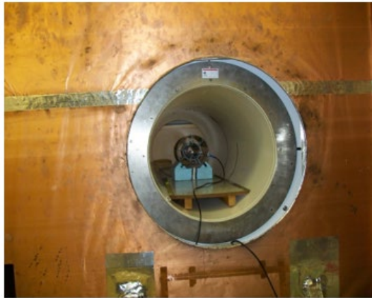
Figure 6: The Field Cycling MRI system used for the study.
