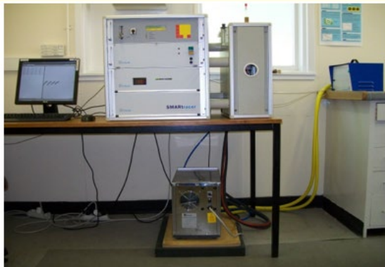
Figure 4: “Stellar SMARtracer FFC relaxometer” and accessories.
