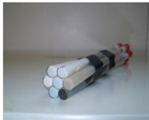
Figure 3: The composite phantom, made up of seven NMR tubes of different sample concentrations.
