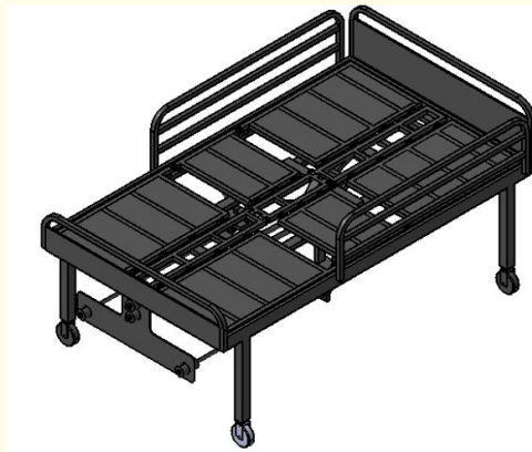
Figure 9: Geometrical model of hospital bed chosen for FEM analysis.
