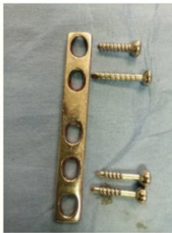
Figure 6: Ulnar side plate: Narrow 4.5 mm plate, signs of re-use, malleolar screws and locking bolt.
