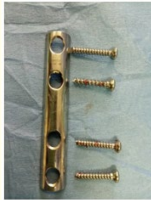
Figure 5: Radial side plate: 4.5 mm Half tubular plate, signs of re-use with 3.5 mm cortical screws.
