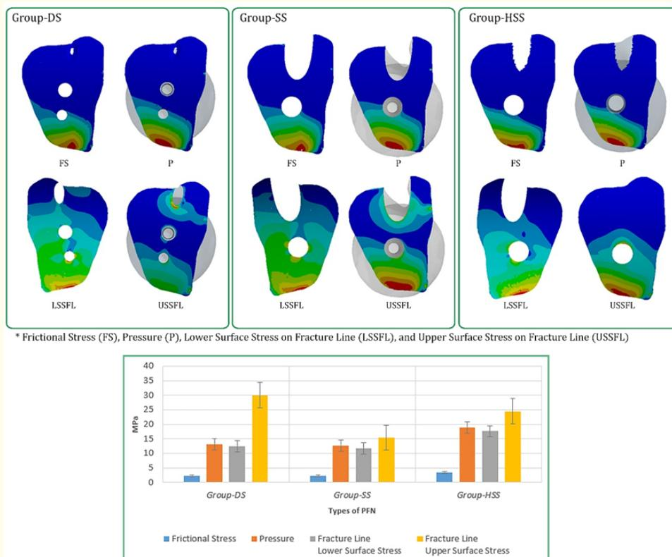
Figure 3: Stress analysis results on fracture line.
