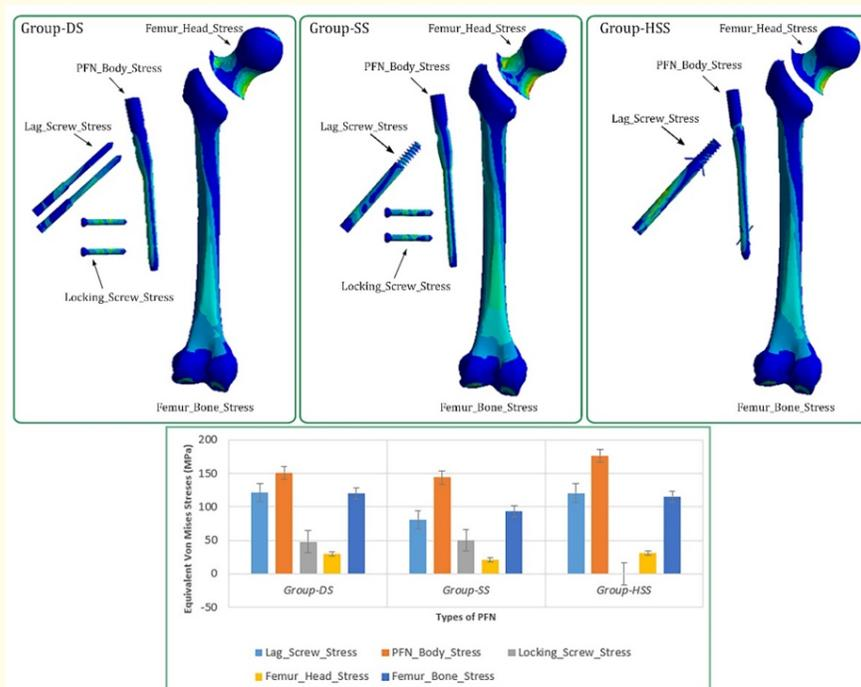
Figure 2: Equivalent von mises stress analysis results of each component of PFNs.
