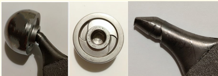
Figure 2: Fretting corrosion of the neck; note the damage at the base of the femoral neck, medially, caused by impact of the female portion of the head.
