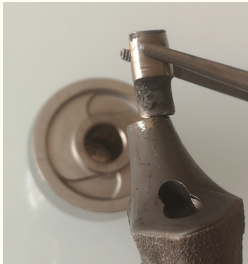
Figure 5: The break-section divided in two parts: the lateral one, curved "crescent-like", horizontal; the medial part was wedge, "cotyledon-like", vertical.
