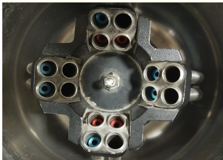
Placement of citrate and plain vials containing autologous blood samples for differential centrifugation (with counter balance)
