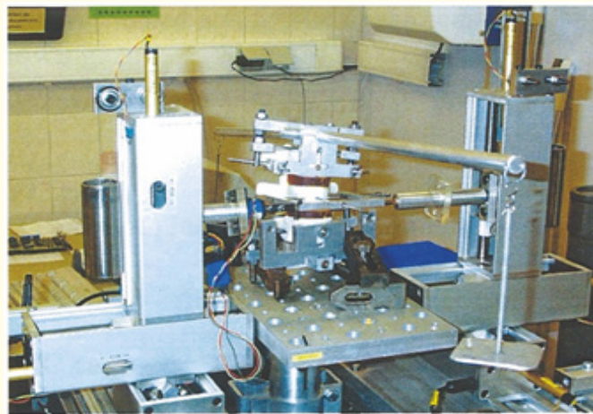
Figure 1: 2TM spine segment testing machine. The test device and protocol are labeled by a quality certification NF EN ISO/CEI 17025.
