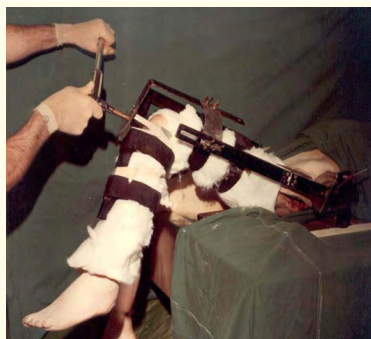
Figure 1: Internal rotation torque being applied when the hip joint was standardized to a fixed angle of flexion and adduction.
