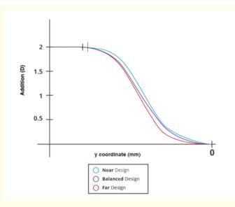
Figure 3: Progression profile for 3 different designs: near, balanced and distance.
