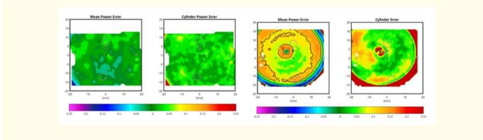
Figure 4: Left, lens correctly manufactured. Right, lens produced with manufacturing errors.
