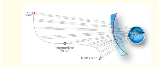
Figure 1: Eye-Lens system model and ray tracing used to compensate patient's vision in a free-form personalized lens.
