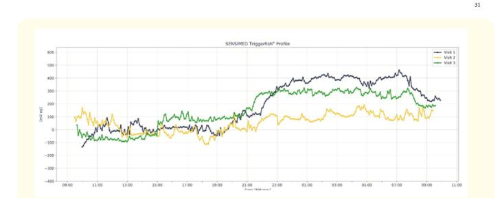
Figure 3: Contact lens sensor output from 3 different recording sessions, showing intraocular pressure-related profiles (blue: first visit [baseline]; yellow: second visit [1 month]; green: third visit [6 months]). At each visit, eyedrops were applied right before sleep, between 21:30 and 22:00.
