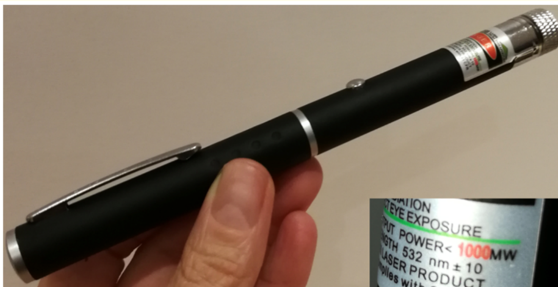
Figure 3: Green laser pointer. Note the high power (< 1000 mW).
