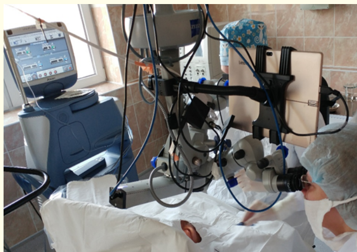
Figure 1: Polaris Keratoscope with tablet PC display, mounted on Zeiss OPMI Visu 200 S8 microscope (under microscope objective using dove tail adapter) during clinical tests at Grodno Regional Clinical Hospital.
