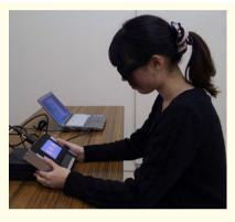
*Figure 1:* High-resolution 3D monitor which we used for a stereoacuity test, and PC for visual target control. Subject is in a state of dichoptic viewing using polarized (circle) glasses.
