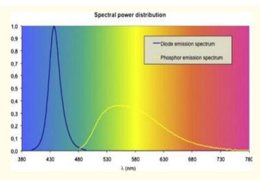
*Figure 1:* Spectral representations of using LEDs and with yellow secondary emission from phosphor, emitting with light. (www.sciencedirect.com, Behar-Cohen et al. (2011)) [4].
