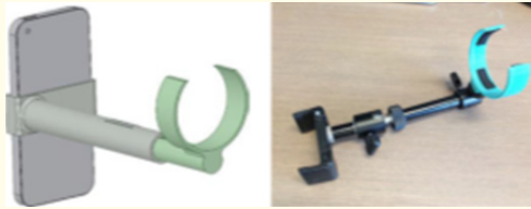
Figure 8: Lens bracket to hold the 20D lens.
