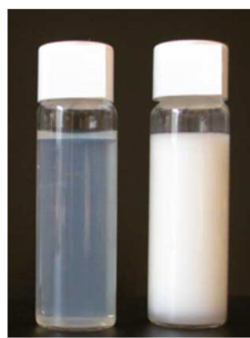
Figure 1: Picture of a nanoemulsion (left) and a macro-emulsion (right) with droplet diameters of 35 nm and 1 \mu m, respectively [3].
