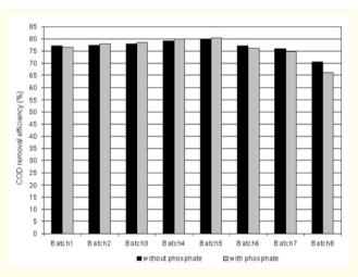
Figure 8: Comparison between COD removal efficiencies with and without presence of phosphate for 24 hours.
