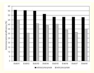
Figure 10: Comparison between Ammonia removal efficiencies with and without phosphate for 24 hours.
