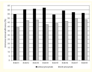
Figure 9: Comparison between Ammonia removal efficiencies with and without phosphate for 6 hrs.
