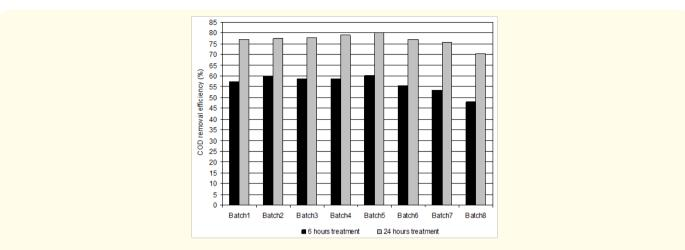
Figure 2: Comparison between COD removal efficiencies of 6 and 24 hr treatment.
