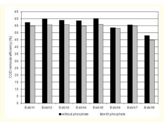
Figure 7: Comparison between COD removal efficiencies with and without the presence of phosphate for 6 hours.
