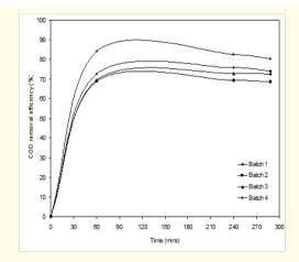
Figure 11: Variation of COD removal efficiency of different leachate systems with time in a bench-scale SBR.
