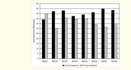
Figure 5: Comparison between Ammonia removal efficiencies of 6 and 24 hours treatment with phosphate.
