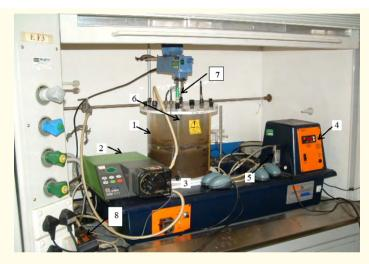
Figure 1: Bench-scale sequential batch reactor. Aerobic Digester W11, (1995) [3].
