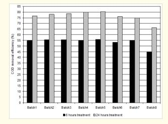
Figure 4: Comparison between COD removal efficiencies of 6 and 24 hours treatment with the presence of phosphate.
