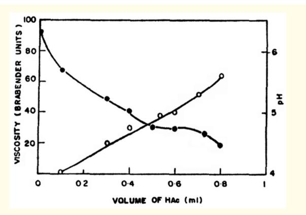
**Figure 1:** Rise in viscosity against weak-acid induced lowering of pH during gelation of shark proteins. Acetic acid was added drop-wise to homogenate of equal amounts of washed shark meat and water. The viscosity change during acidification was determined by Brabender visco-amylograph. Reprinted from Venugopal., et al. (1985), with permission from Elsevier.
