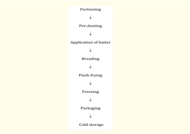
Figure 5: General process flowchart for the production of coated products.
