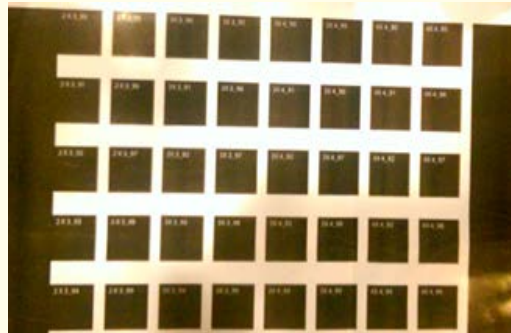
Figure 7: The digital test form was composed of a solid plain area and 4 groups with different feature size, No.1 (2x3), No.2 (3x3), No. 3 (3x4), and No. 4 (4x4) and each group with intensity changed from 90% to 99%.
