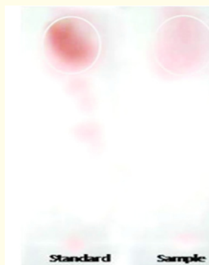
Figure 2: Thin layer chromatogram of bacterially sized IAA detected by Salkowski's reagent compared with standard [15].
