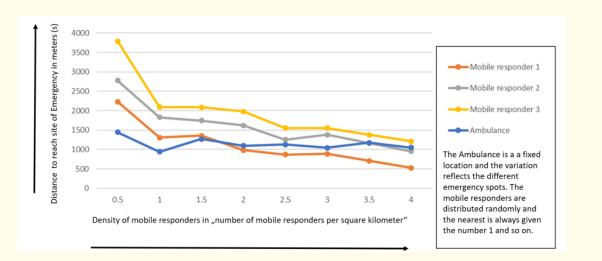
Figure 2: Case Study simulation outcome - with each data point calculated as average of 10 rounds of simulation: distance depending on density of mobile responder and vehicle.
