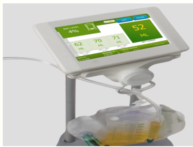
Figure 1: BD Sensica. Urine is measure when it comes into the foley bag, on the scale.
