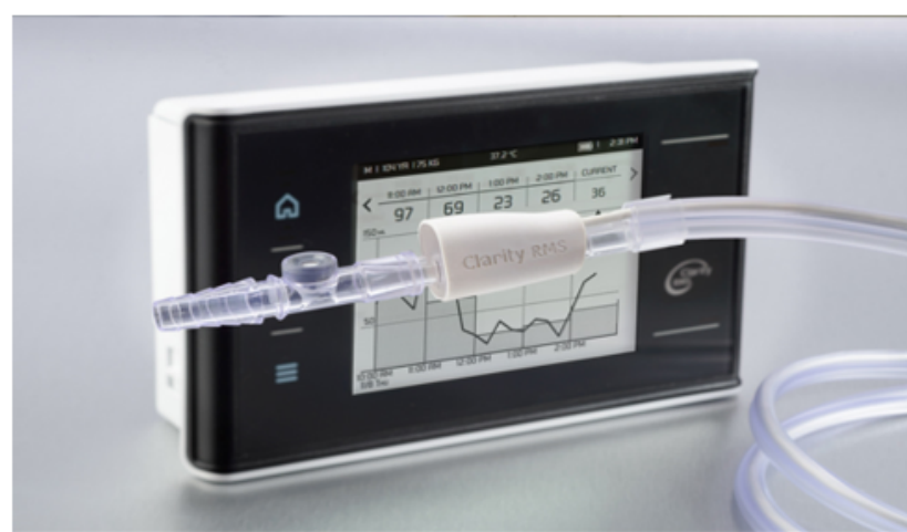
Figure 3: Renalsense clarity. Urine is measured as it comes out of the foley catheter via a flow sensor.
