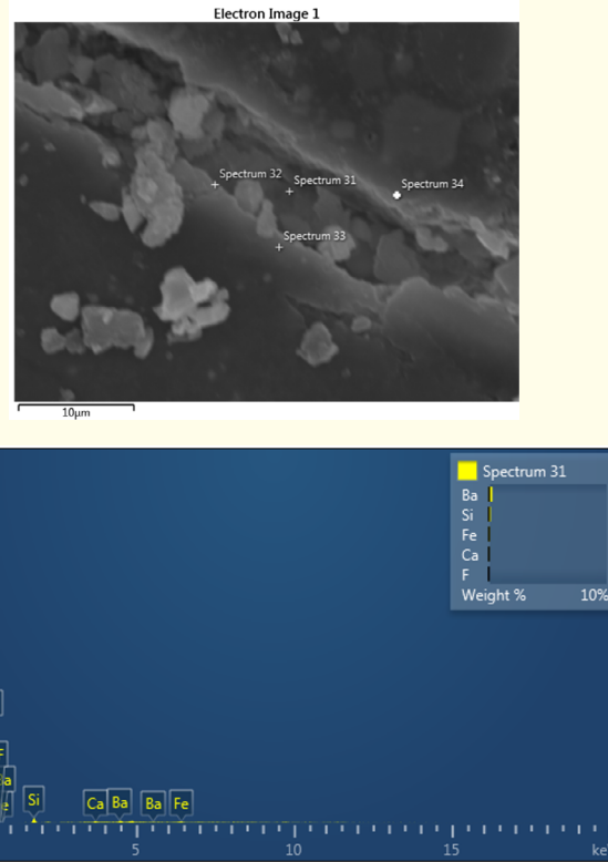
Figure 4: Silane treatment with Ceramic Primer Plus for 20s on IPS Empress II (e-max) with ED Primer II for tooth dentine and cementation Panavia F 2.0 (Spectrum Point Elements Analysis).
