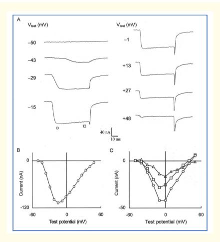
Figure 1: A) Whole cell  $Ba^{2+}$  currents recorded from a LYC neuron in Lymnaea stagnalis held at -70 mV and step depolarised for 70 ms to the test potentials indicated next to each current trace. (B) I-V curve of peak amplitude of currents in 'A'. (C) I-V curves for peak ( $\bigcirc$ ), sustained ( $\square$ ) and transient ( $\triangle$ ) current measurements recorded from a different LYC, step depolarised for 150 ms at each test potential in 10 mV increments.
