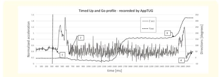
Figure 1: One accelerometer and one gyroscope as captured by AppTUG. The vertical dashed line indicates the Start signal. We can notice the stand-up time (SUT) between 1 and 2, each step in either direction, rotation circa 1.5 seconds, and sitdown time (SDT) between 3 and 4. Data is sampled at 100Hz, time is in milliseconds.
