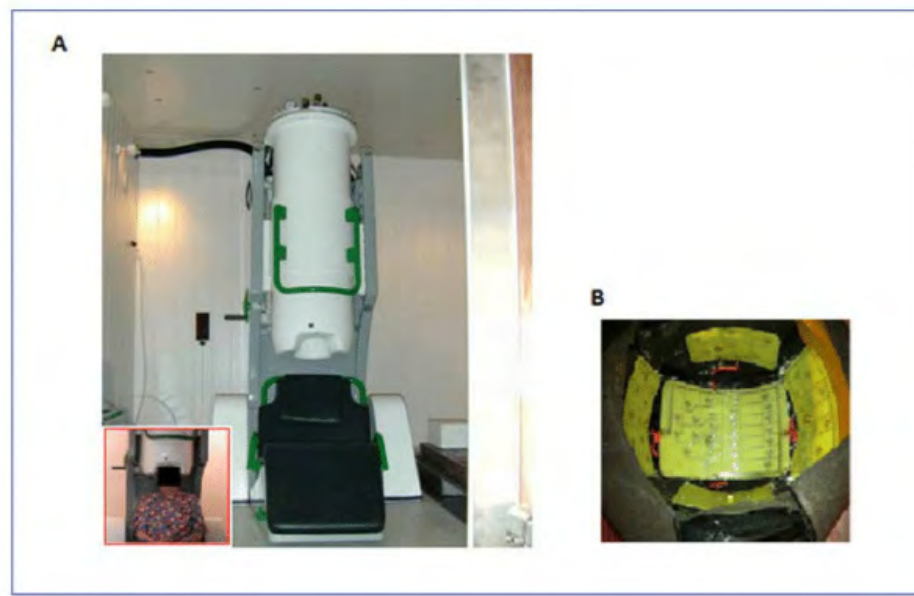
Figure 1: A) The 122-Channel MEG System; B) the pT-TMS Electronic Device.
