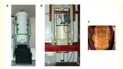
*Figure 1: A*) The 122 channel MEG system inside the shielded room *B*) The one channel MEG system inside the shielded room. *C*) the configuration of the stimulation coils within the helmet of the electronic device.
