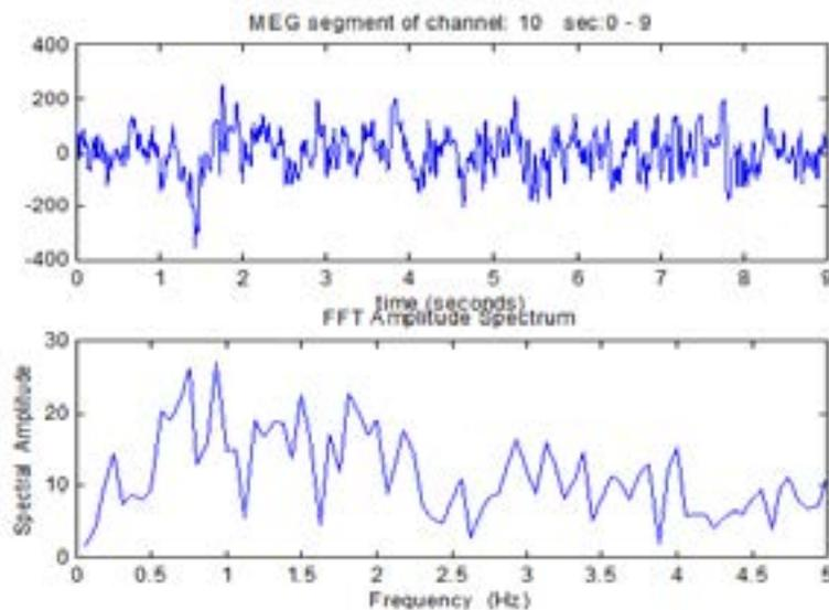
**Figure 2:** This figure is shown the MEG record of 9 sec obtained from a dystonia patient with reference number 2. Application of FFT on the above MEG record we get the primary dominant frequency in the 2 - 7Hz which is in the range of 2.9 Hz.
