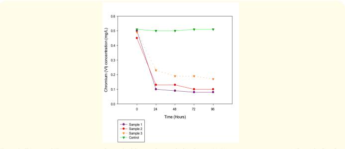
Figure 3: Chromium(VI) concentration within each of the samples as calculated using OD540nm measurements every 24 hours for four days.
