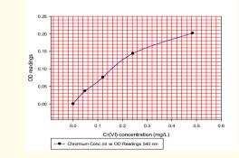
Figure 1: The standard curve that was plotted to show the OD readings for known Cr(VI) concentrations.
