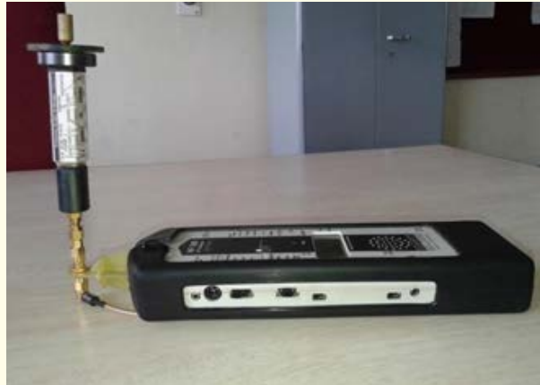
Figure 2: Radiation measuring device HF59BTM and isotropic antenna.
