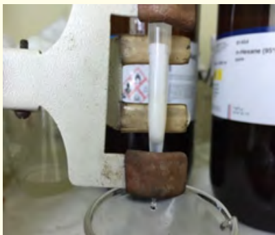
Figure 5: (B) Silica gel column with the sample being collected.
