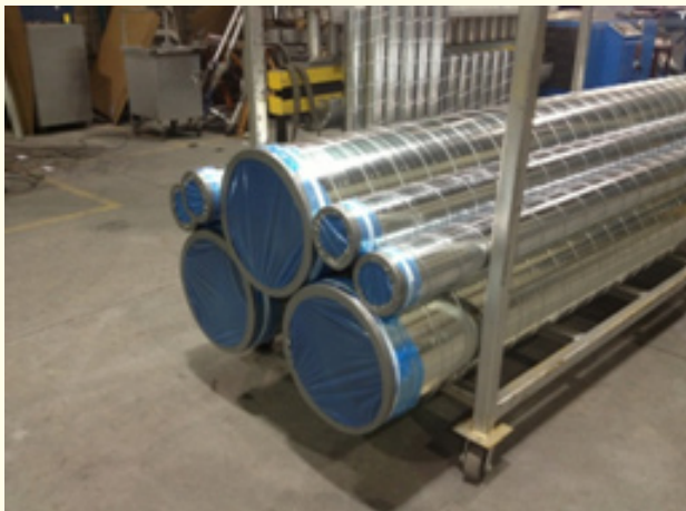
Figure 2: Sealing of openings of duct by plastic foil.
