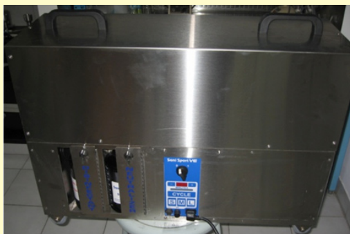
Figure 1: Ozone generating apparatus "HYGIENIST" (Sani Sport, Montreal Canada).
