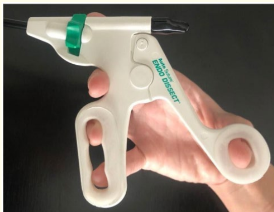
Figure 4: Forceps handle and hand model for grip adapters design. Image with grip adapters on.
