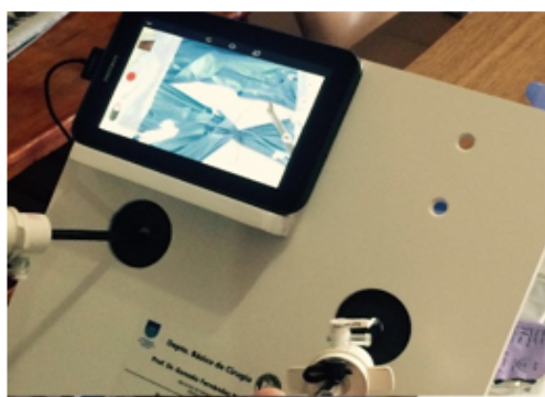
Figure 3: Front view of the simulator with the tablet as interface and with the app on camera mode, recording training session.
