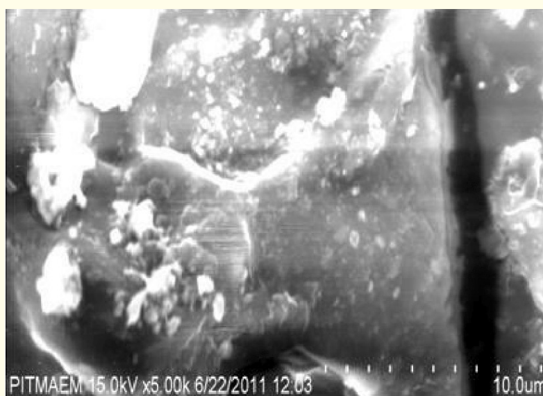
Figure 3a: SEM structures of the optimized batch [NiPAAm-1] inner surface in dry state.
