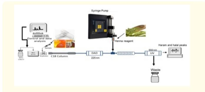
Figure 1: Developed on-line HPLC-henna staining halal gelatin protein detection methodology.
