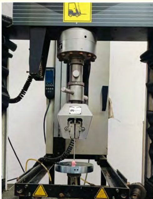
Figure 1: Compressive strength assessment in which each sample was placed with the flat ends up between the plates of the universal testing machine (Instron).
