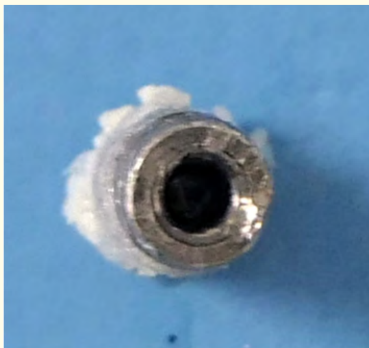
Figure 5: The extracted implant showed its upper side damaged by the failed attempts to remove the cover screw.
